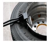
Hold tool by straight handle. Let bent handle drop away. Insert roller between rim and bead by pushing on foot pad. Make sure rim is in notch on tool and roller is under top bead.
