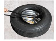
Pull the bent handle down to remove the top bead from the rim.
