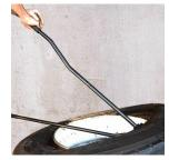
Pull the straight handle over and down to lift the top bead. The straight handle should now be resting on the rim.
