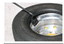
Insert bottom bead tool between edge of rim and bottom bead.
