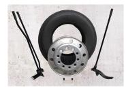
Continue to rotate the handle to completely remove the tire from the rim.
