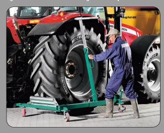
Top-point wheel connection rod keeps the wheel in safe balance.
