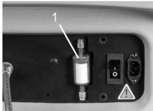
Fig. 34: Refrigerant identification unit
